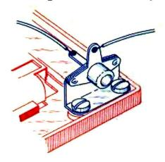
Under the screw at 5 there are now two wires. This is enough, so tighten the screw firmly.
