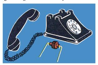
coils generate a magnetic field which goes through your pick-up coil. These magnetic fields in turn generate little voltages in the pick-up coil, which are further amplified by the monitoring set until they reach loudspeaker volume. Find out by trial and error what the best position of the pick-up coil is. With some telephones which are shielded very efficiently, this trick might not work.
