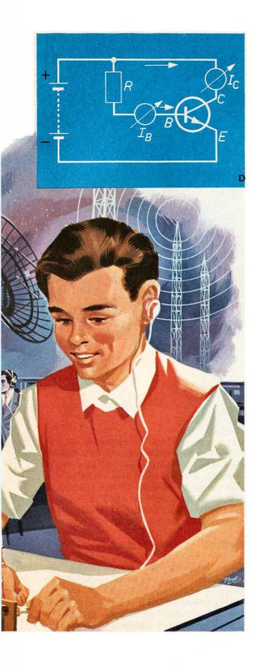
speaker. If one transistor does not give enough amplification, we can use two or even three, one after the other ("in cascade").
