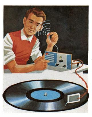
and fro. If you attach a diaphragm to this slab of Rochelle salt, the diaphragm will start to vibrate and you hear a tone. The opposite is possible too. When sound sets the diaphragm vibrating, the Rochelle salt slab is bent backward and forward and a voltage is generated between the two conducting layers on the slab. Used in this way it is called a crystal microphone.
