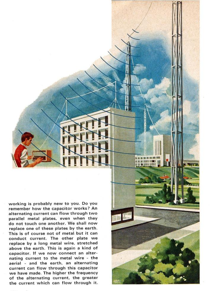
Now we have already said that what we call an electric field is generated between the two plates of a capacitor. This happens here too. Between the aerial wire and the earth an electric field is generated, but that is not all. You know that a magnetic field is emitted from a coil when a current flows through the coil. This is also true of a straight wire, so that a magnetic field is generated about
